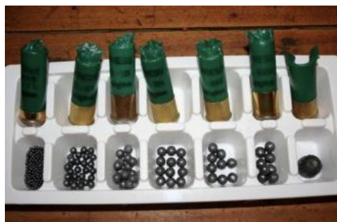
↑ Cartridges displaying a range of metal projectiles. © Omega Research Foundation
