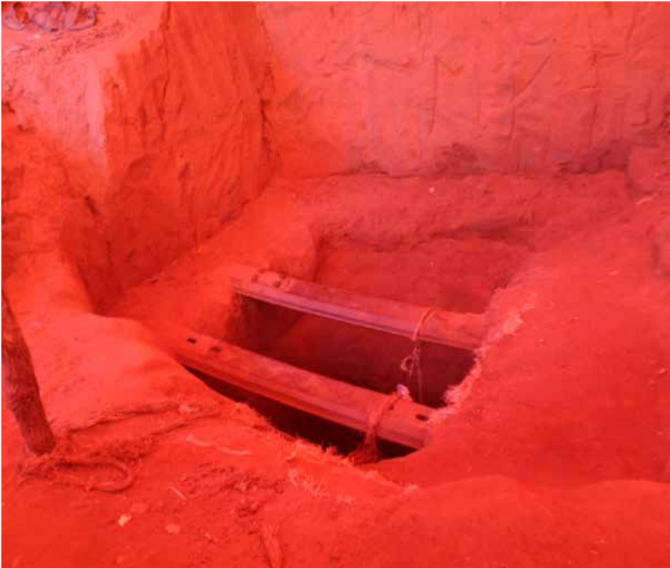
Miners use a rope attached to a beam stretched over the pit as support to climb down into and out of the pit, Kasulo, March 2017 © Amnesty International/Afreview
