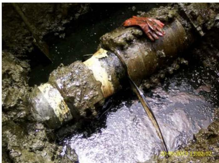
In another case, a spill occurred at Ikarama in Bayelsa state on 24 May 2013. The JIV, which took place on 30 May, six days later, found the spill was due to a hacksaw cut.<sup>64</sup> However, the photograph (reproduced above, taken from Shell's website) does not show a hacksaw cut. According to Accufacts: "Most likely this photo suggests that the seal on a previous clamp repair has failed for various reasons, such as poor installation."<sup>65</sup>
