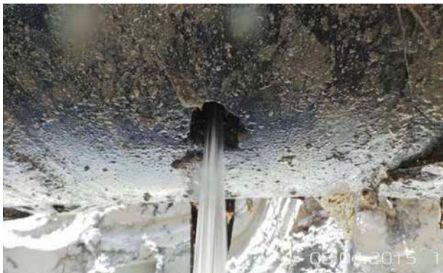
Leak point at Eni's 24" Ogoda/Brass pipeline (2015) . Eni photograph.
