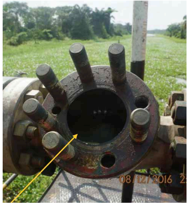
Close up of Shell's Benisede Well 6S Wellhead at Ojubo, where the company said unknown persons had stolen a "surface safety valve" causing a spill on 30 November 2016. Shell photograph.
