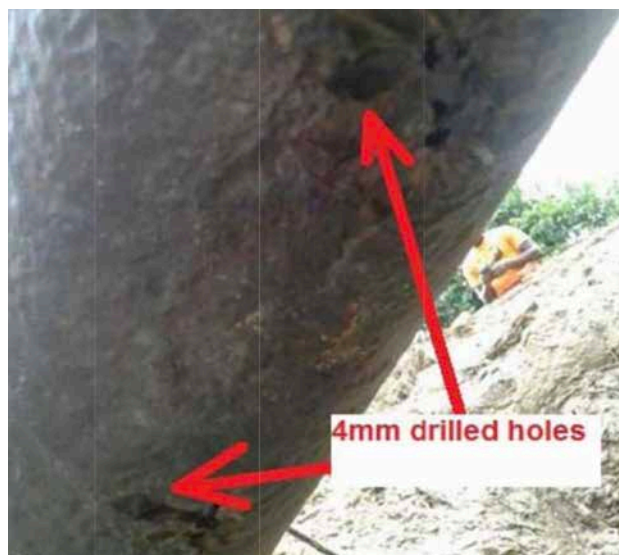
Leak point at Eni's Obiafu 26ss Flowline (2016). Eni photograph.
